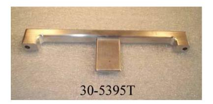
This unique Signet tool makes it much easier to install the extraction assembly in the source housing on the CF/DF3000, 350D/DE and 300XP Varian Medium Current Implanters. If the extraction assembly is not installed in the center of the source housing the motor adjust may not have enough travel for optimum beam adjustment. This tool makes the correct alignment quick and easy.
