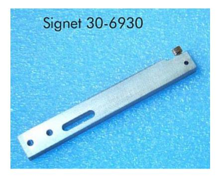
This improved design uses a Tantalum Screw in a Molybdenum Filament Connector. Signet Products developed this design concept in the early 1990's which is based upon tantalum's expansion being greater than molybdenum's as the temperature increases. Our design replaces the old "tuning fork" filament clamp that loses its grip over time. This material combination results in longer filament clamp life, easier filament installation and improved electrical continuity at the filament interface.
