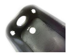
The spent arc chamber box liner above was in operation for more than 1500 hours before eroding through. During that time eleven sources were rebuilt.
