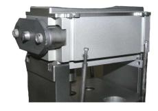
A photo of the complete OEM Arc Chamber Assembly. Note complicated repeller assembly requiring 13 parts most of which are unique to the ultra source.
