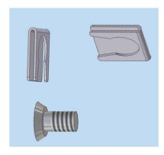
You can see in the drawing above that a little of the bottom of the screw head has been machined off to accept the Screw Shield that just clips on.
